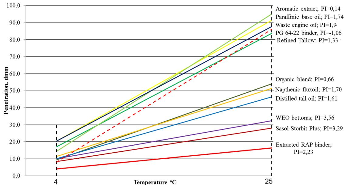
**FIGURE 1 Penetration Values at 4°C and 25°C and Penetration Index (PI) of Rejuvenated Asphalt.**
