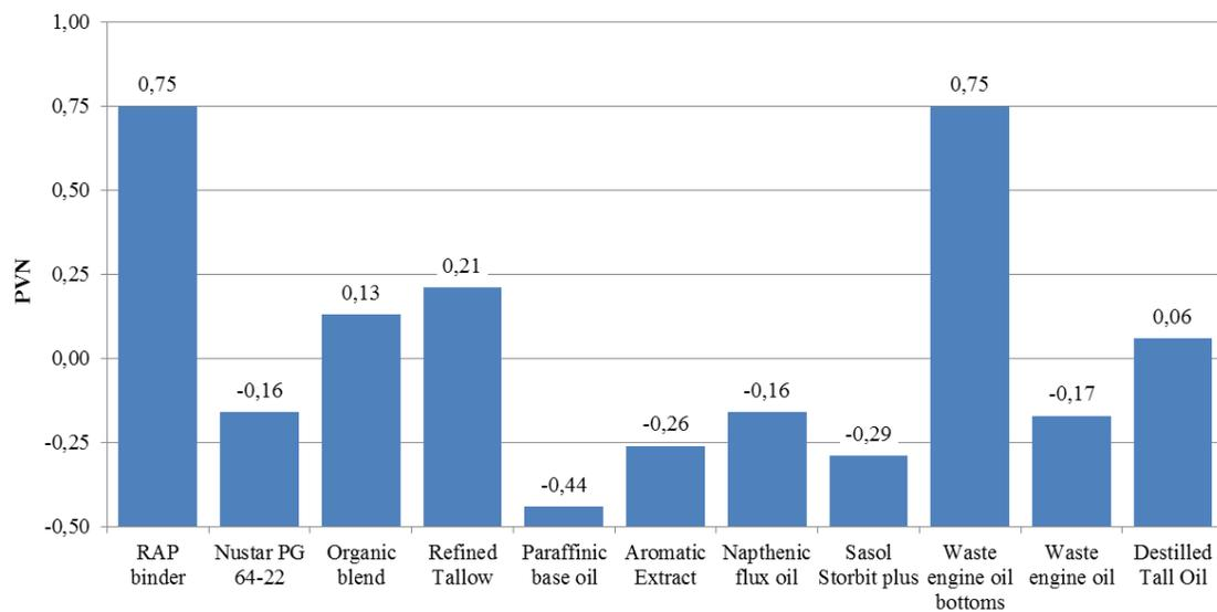
**FIGURE 2 Penetration Viscosity Number (PVN).**
