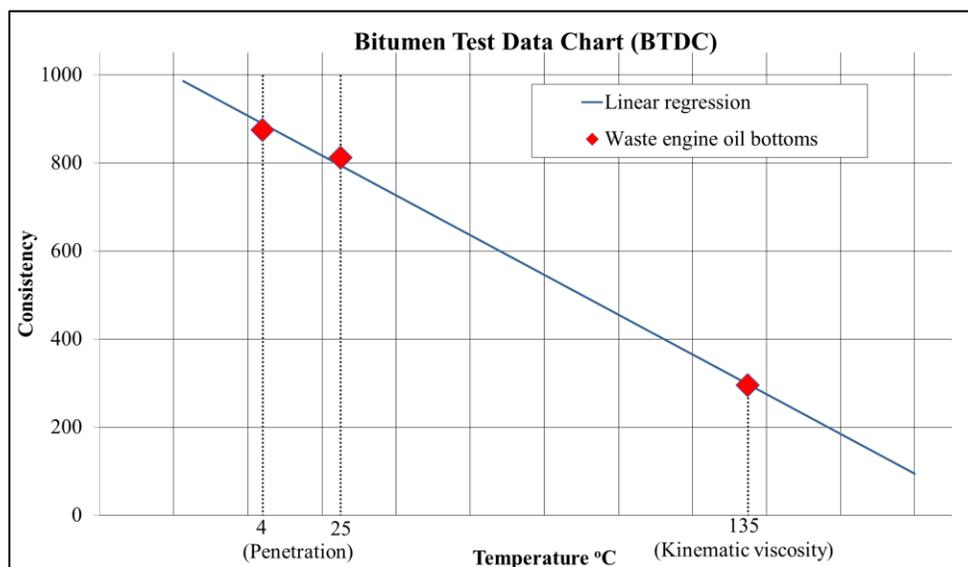
**FIGURE 3 Bitumen Test Data Chart (BTDC) Example for WEO Bottoms.**
