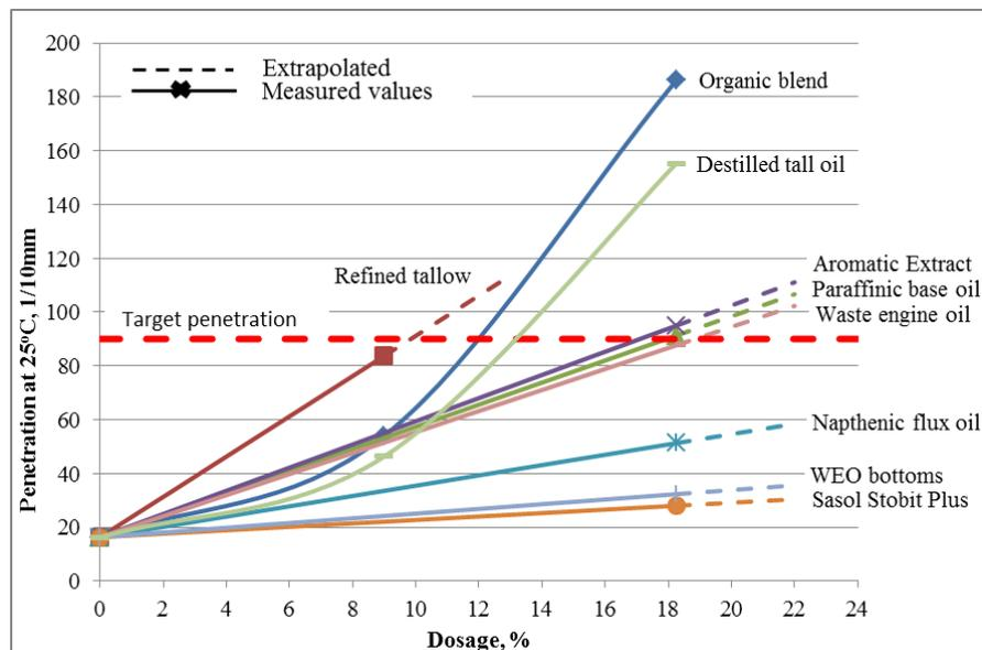
FIGURE 4 Required Dosage to Reach Target Penetration at 25°C.
