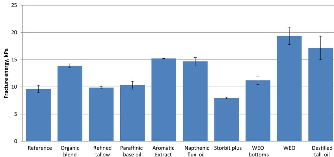
**FIGURE 7 Fracture Energy.**
